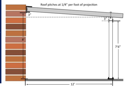
Take the measurement from the deck / patio to the bottom flange of the installed C Channel. For the purpose of this illustration, call it 8 feet. With a pitch of 1/4" per foot of projection, the total height of the post & beam assembly will be 8' minus 3"  $(12 \times 1/4$ ") = 7' 9". The beam in this illustration is 3" tall which means the 8' post supplied with the kit would need to be trimmed to a finished height of 7'6".
