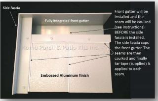
It is possible you will get our premium side fascia / front gutter assembly. As you can see below this side fascia is assembled with the flange down so as to cap the premium front gutter. You will need to trim about 3 1/2" from each flange on the end that caps the gutter to make a nice snug fit.
