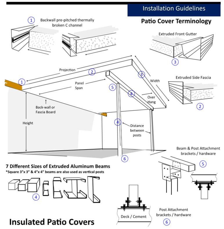
3", 4" or 6" thick "snap lock" Insulated panels
