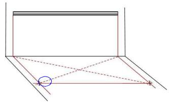
the height that you have determined as per the instructions in Step 3. (Do not do this on a windy day!). You can "square" up the awning perimeter by snapping chalk lines off the ends of the rear C channel installation, down the wall and plumb to the deck or patio surface. Run another chalk line perpendicular from that line on the wall out along the surface of the decking or patio.
